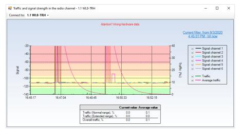
different frequency Select channels one by one and try to identify the one with the lowest noise level and the least amount of peaks on the graph (which correspond to radio signals). The number of this will channel need to be specified **EK-WL8-TRH** in properties (described further in this manual).
